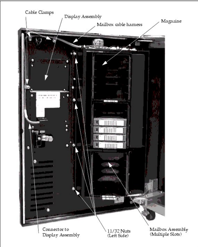
Figure 5. Installing the Multiple-Slot Mailbox Assembly
